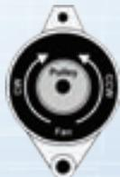
**\* ALTERNATORS WILL CHARGE WHEN TURNING IN EITHER DIRECTION**
