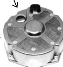
Delco style alternators use flame arrestors instead of sealed brush compartments.
